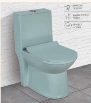
LUMINA-S&P OLIVE (Matt) L 690 W 375 H 750 S Trap - 225mm(9") P Trap - 175mm 46 Kg.
