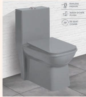
EVORA-S&P SMOKE (Glossy) L 660 W 360 H 750 S Trap - 225mm(9") P Trap - 190mm 48 Kg.
